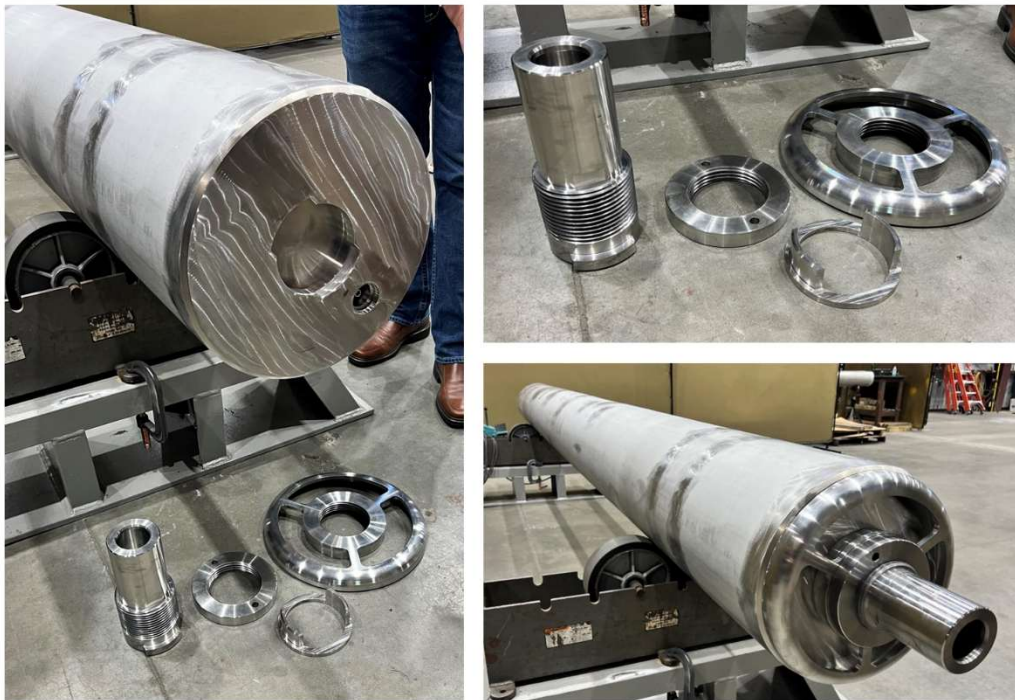
Figure 3. UCS Prototype, with lift adapter assembly fully disassembled (left), disassembled lift adapter assembly (top right), and fully assembled prototype canister (bottom right).
