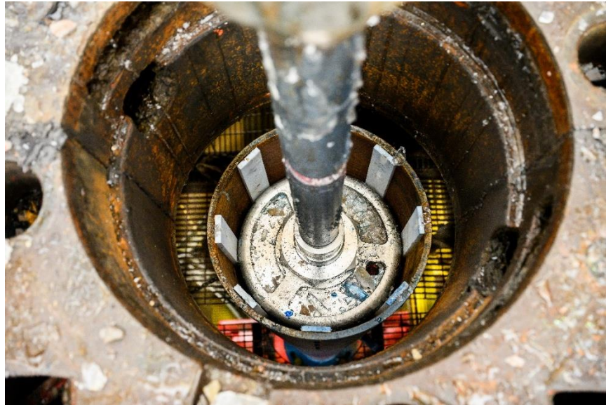
Figure 2. Successful emplacement and retrieval demonstration of a full weight and size disposal canister in Cameron, Texas.
